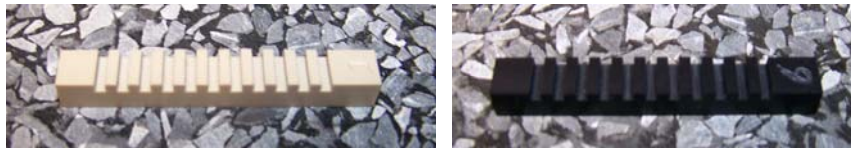
Figure 2: PEEK (left) and PPS with 40% glass (right) step gauges
