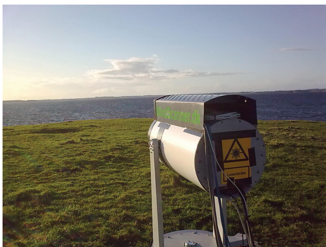
Figure 2: The scanning lidar measuring upwind towards the cliff of Bolund. See figure 1.
