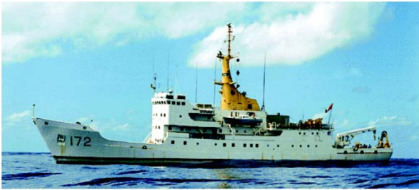
Fig. 2: The Canadian Navy research ship CFAV Quest. ( L = 71.6 m, B = 12.8 m, T = 4.8 m, C_p = 0.51 )
