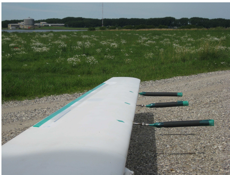
Figure 4.6: Photo of the V27 blade before being mounted on the turbine. The trailing edge flaps, the Pitot tubes and the pressure tabs are protected to avoid any damage during the installation and intrusion of water in the Pitot tubes and the pressure tabs.
