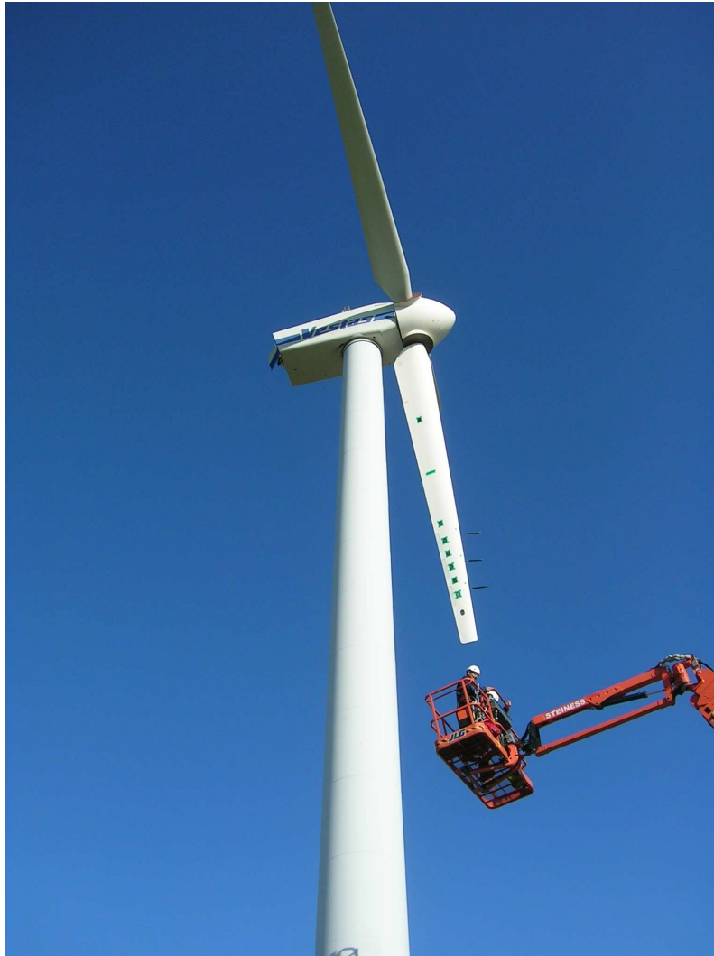
Figure 4.7: Photo of the V27 demonstrator turbine. Before running the tests, the rotor is locked with the blade with trailing edge flaps pointed downwards in order to allow access to the blade for checking the actuators and sensors, and remove the protections.
