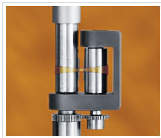
Figure 2: The Sentmanat add-on device to traditional shear rheometers from Xpansion Instruments.
