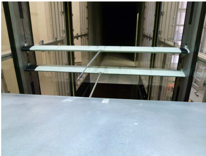
Figure 2. Slanted hot-wire holders set-up
