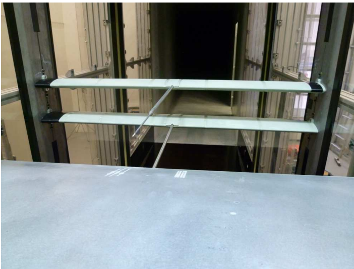
Figure 2. Slanted hot-wire holders set-up
