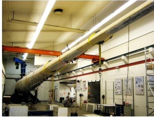
Fig. 2. The blade bolted to the test rig. The tip was truncated at 25m. The blade is loaded at a 30^\circ angle to the flapwise direction, simulating combined flap- and edgewise loads.
