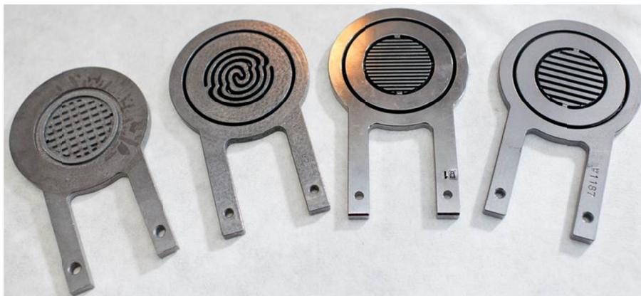
Figure 4.5: Photograph of the four machined flow patterns. The diameter on all the flow areas is 35.7 mm. ©fagpress
