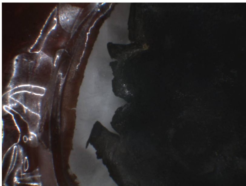
Figure 6.6: Photograph of membrane after disassembly of PBI-MEA8 after electrolysis test.
