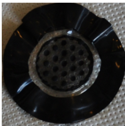
Figure 7.4: LIQ-MEA3 disassembled after electrolysis test. The electrode diameter was 38.5 mm.
