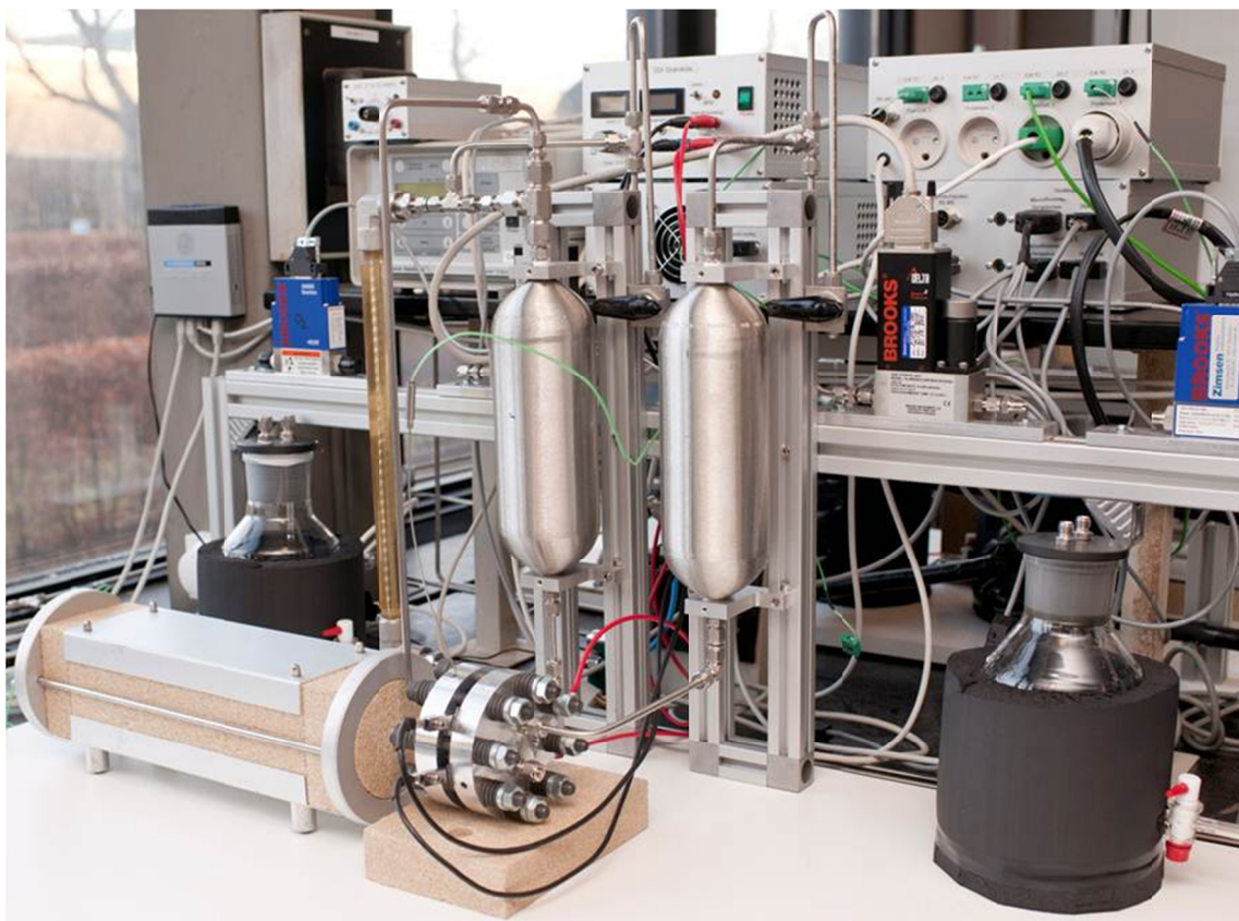
Figure 4.7: Photograph of the pressurised electrolysis system. ©fagpress
