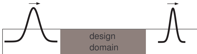
Figure 3. Design problem. A single gaussian pulse is to be compressed when propagating through the design domain by a suitable stiffness and mass density distribution in space and time.
