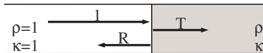
Figure 1 - A one-dimensional acoustic wave in air is partially reflected ( R ) and transmitted ( T ) at the interface to an acoustic medium.
