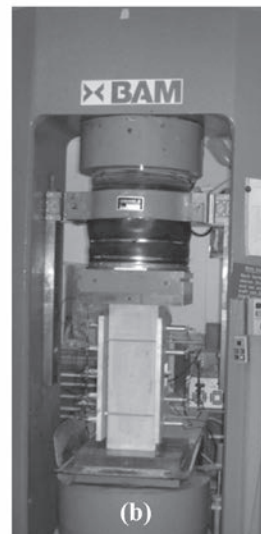
Fig. 2—(a) Arrangement of mounted sensors for surface wave velocity measurement in Experiments I and II; and (b) Specimen I being loaded in 2 MN (450 kip) loading machine.
