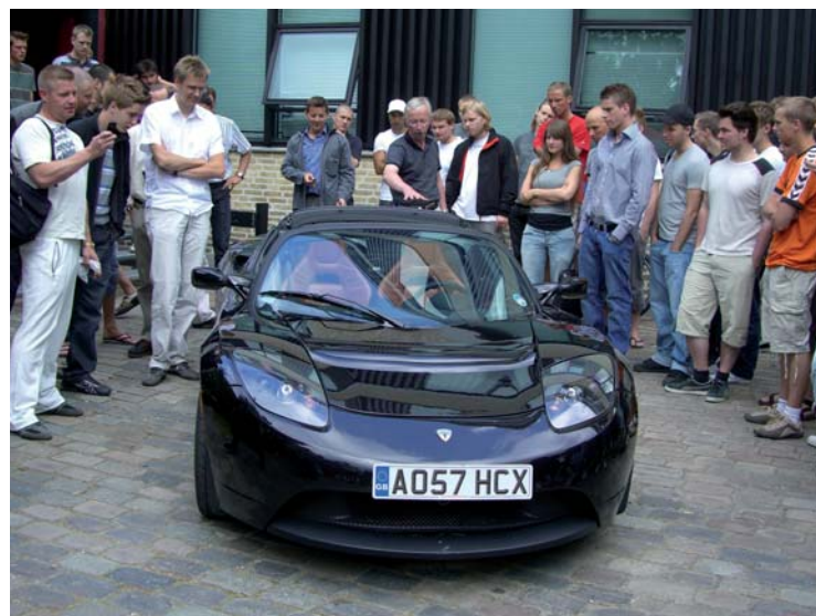
Fig. 12.6. Students and employees from the DTU Centre for Electric Technology examine the Tesla Roadster (pure electric, 0-100 km/h in 4 s, 250 hp, >200 km/h, 360 km per charge). Today electric cars can be compared with conventional cars based on internal combustion engines.
