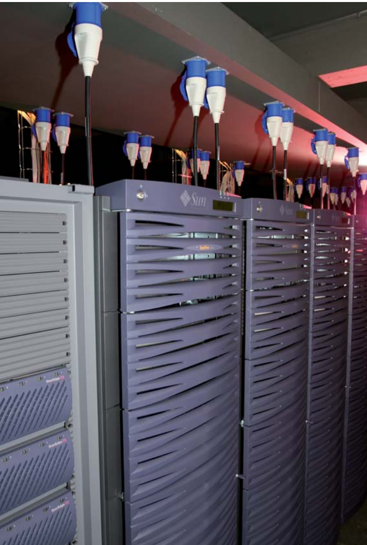
Fig. 9.4. DTU's High-Performance Computing Installation currently consists of two symmetric multiprocessor computers with 96 dual-core processors in total and more than 600 GB of memory
