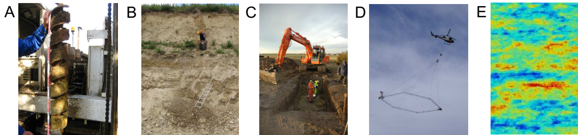
Figure 3.1: Characterization methods for geological heterogeneity. The pictured methods were employed in Denmark to record sand deposits in clayey tills. They are in particular: A borehole logging, B outcrop mapping, C excavations, D airborne geophysical surveys, and E stochastic simulation.
