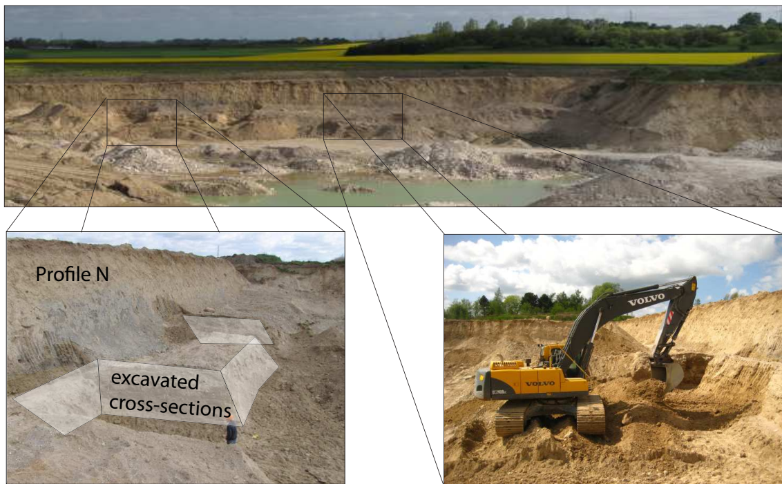
Figure 3.2: Excavation in the Kallerup gravel pit. The images show the Kallerup profile N and the excavation of smaller cross-sections. These were used to measure and map sand lenses at small scale.
