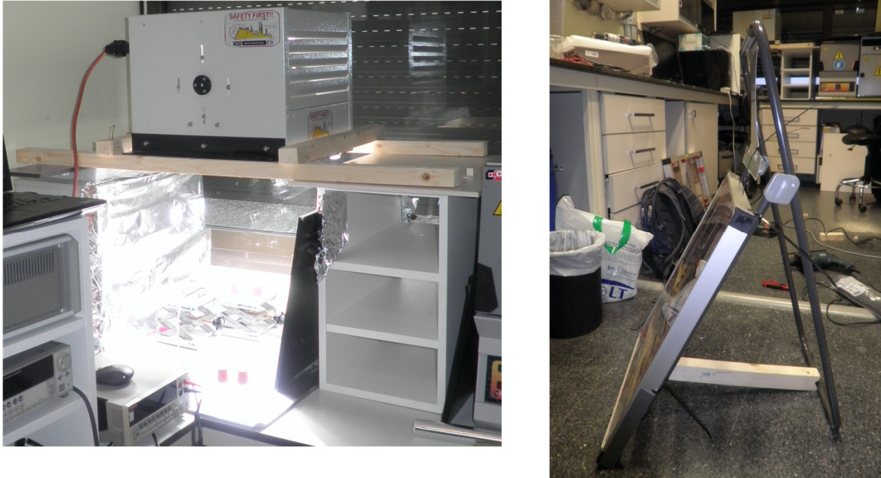
Figure 4.5 left: The construction of a wooded frame in a Barcelona created enough space for the panel to be measured under their sun simulator. right: the panel in Barcelona attached to a simple rack for paper towels.
