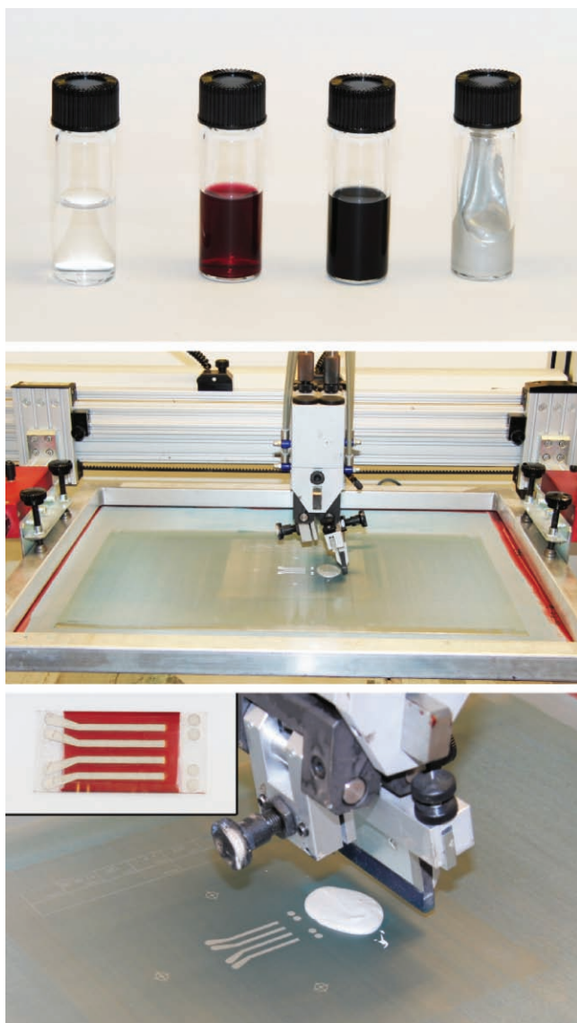
Figure 2. Top: picture of the inks involved in the ‘all water based processing’. From left to right: aqueous ZnO precursor solution, aqueous solution of polymer 1 (diluted in order to show color), aqueous PEDOT:PSS with isopropanol and aqueous silver paste. Middle: Picture of the screen printing machinery. Bottom: Close-up of the screen printing process. The silver paste has been applied and is ready to be pushed through the pattern of the mask by sweeping the squeegee across the steel mesh screen. Insert shows a picture of the final device after encapsulation.
