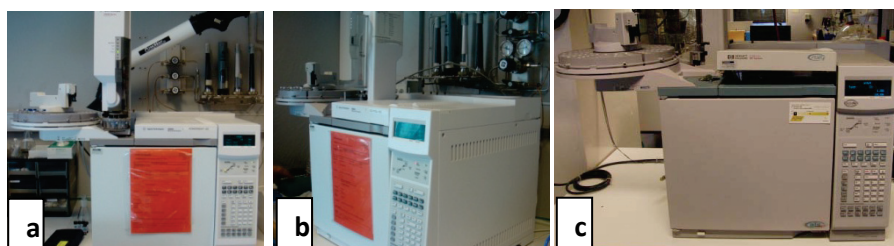
Figure 5.5: Chromatographs used for phase analysis: (a). condensate GC used for analysis of traces of hydrocarbon in MEG phase (b). Glycol GC used for analysis of traces of glycol in hydrocarbon phase (c). Sim Dist GC (which can be) used for analysis of traces of condensate heavier than C 15 .
