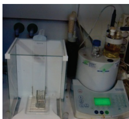
Figure 5.6: Karl Fisher coulometer used for the measurement of water content in hydrocarbon phase.
