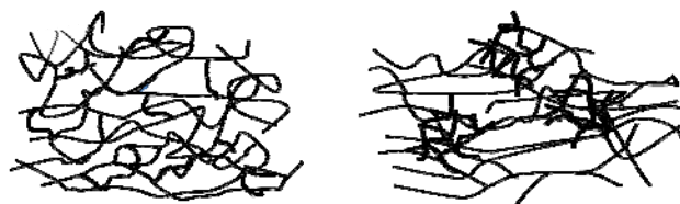
Figure 1a. Schematic illustration of a bimodal network with a non-controlled distribution of the short polymeric chains
