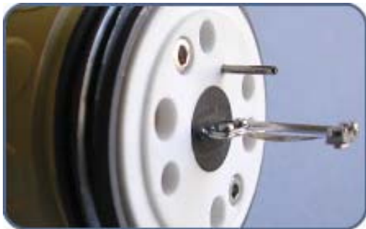
Ohmic heating using platinum foil (14 x 3 x 0.03 mm)
