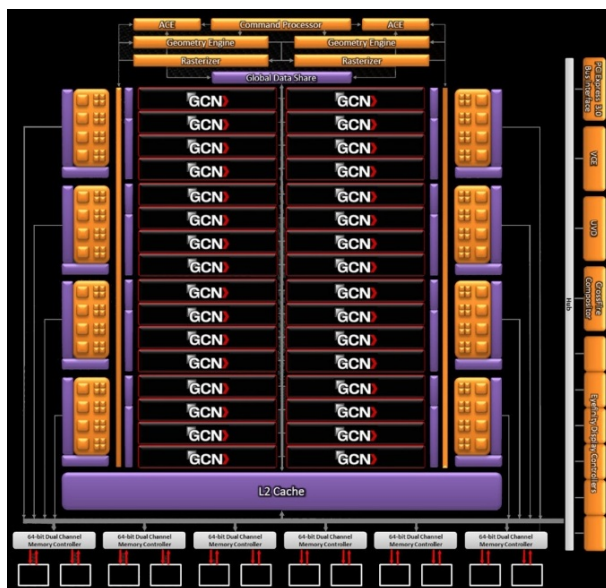
Figure 10.2: [27] Schematics of the GCN based AMD HD7970 GPU.
