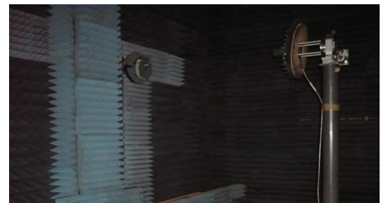
FIGURE 10: Measurement of a rectangular-horn antenna in a planar near-field range.
