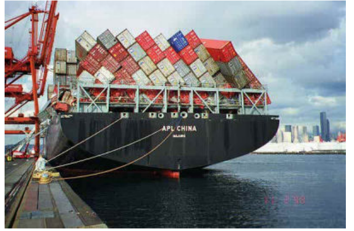
Fig. 1. Devastation of on-deck containers after the APL China underwent parametric roll resonance. ( http://www.cargolaw.com/ )
