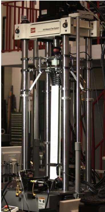
Figure 14 Test setup for experiments on composite beams.
