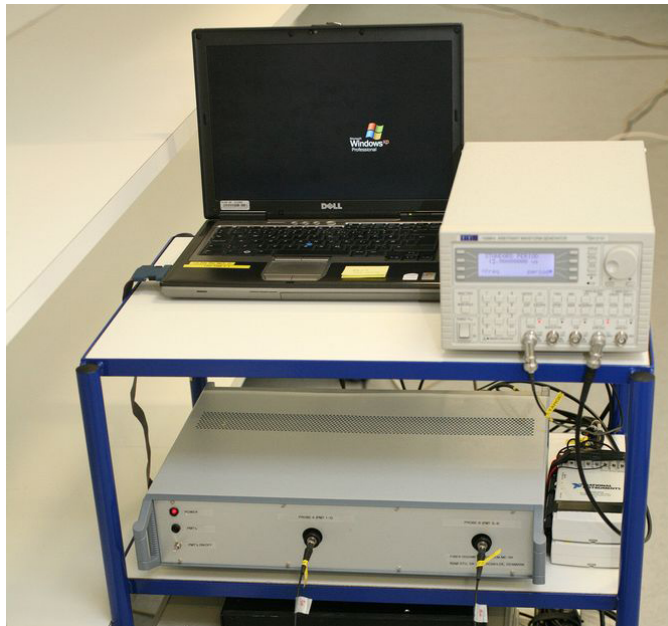
Figure 3.3: ME04 hardware during data acquisition at Rigshospitalet. On the top shelf stands a laptop PC, used for controlling data acquisition and analysis, and a TTI TGA12101 waveform generator used for processing the target current signal from the linac. The ME04 system is seen on the bottom shelf, along with two NI USB-6218 DAQ cards used for data acquisition.
