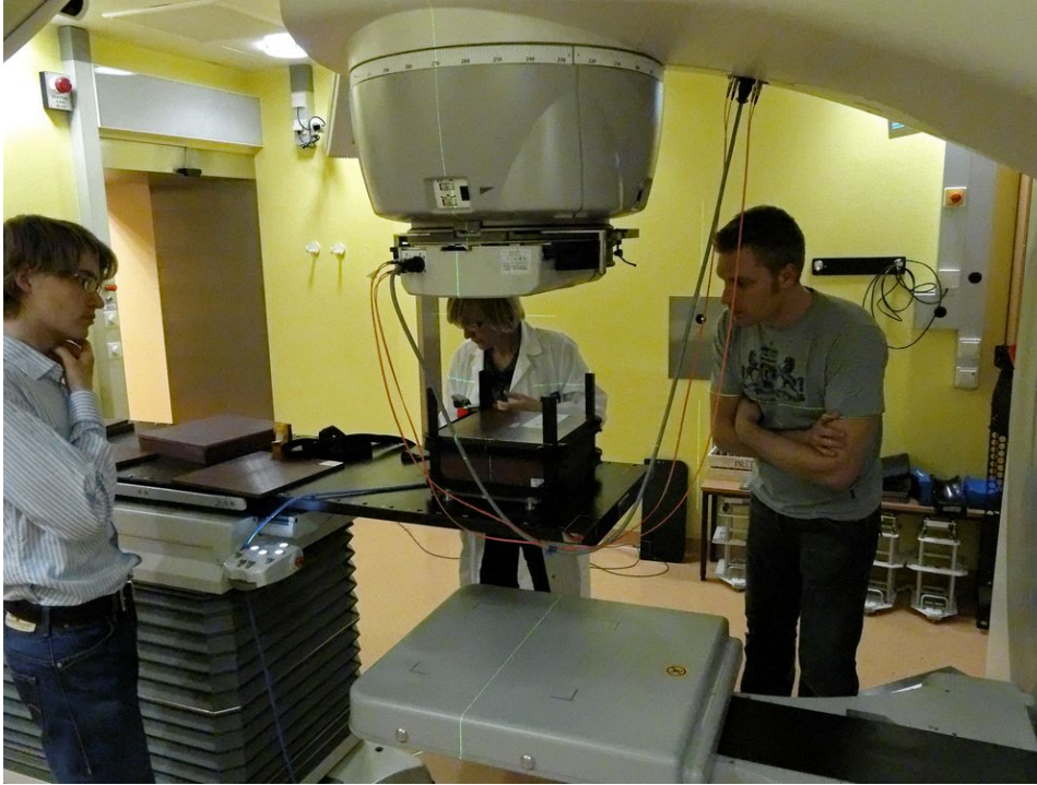
Figure 6.3: Measurement setup at AKH. The dosimeters were irradiated in solid water using 6 MV x-rays from an Elekta Precise ® fitted with Brainlab M3 ™ \mu MLCs. The improvised fixation mount for the phantom was used to minimize alignment errors.
