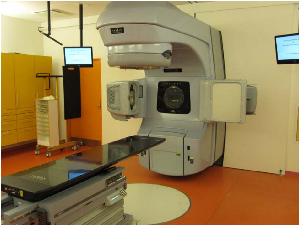
Figure 1.1: A Varian Clinac ® 2300 iX medical linac at the Division of Radiophysics, Herlev Hospital. The machine can deliver x-rays and electrons of different energies, and is equipped with kilovoltage and megavoltage onboard imaging for image guidance during treatment.
