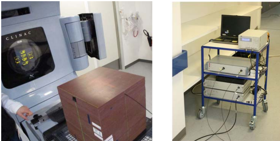
Figure 3.8: Example of measurement setup at Rigshospitalet. Left: Fiber-coupled organic scintillators are irradiated in solid water using 6 MV x-rays from a Varian 2300 iX medical linac. Right: The light signals are transmitted to the detection system on the other side of a concrete maze. On the table (top to bottom shelf) is a laptop for data acquisition, a frequency generator for handling the target current signal from the linac, an ME04 detector system for organic scintillator probes, and two ME03 systems for \text{Al}_2\text{O}_3:\text{C} probes.
