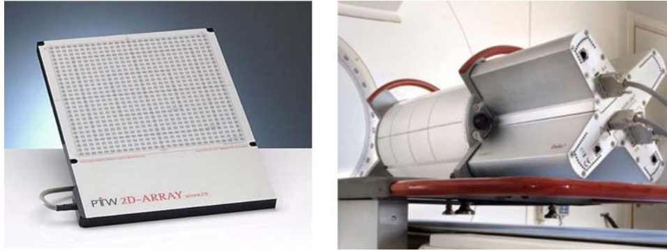
Figure 1.6: Two examples of commercial point dosimeter 2-D arrays for IMRT verification and QA. Left: PTW 2-D ARRAY seven29 ® ionization chamber array, comprising 729 cubic chambers. Source: http://www.ptw.de . Right: Scandidos Delta4 ® , consisting of 1069 p-type diodes arranged in a cross-plane configuration in an acrylic cylinder phantom. Source: http://www.scandidos.com .
