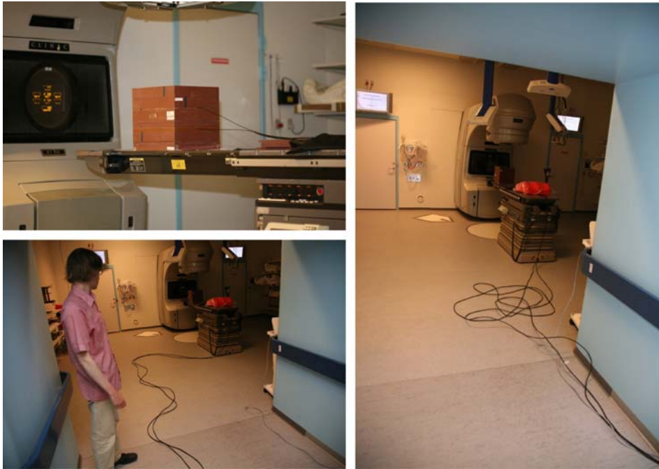
Figure 4.10: Stray radiation-induced stem signal variation by placing varying lengths of fiber in the treatment room during irradiation.
