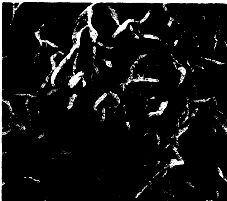
Fig. 11. Scanning electron micrograph showing the surface of a mechanically manufactured magnesium particle.
