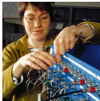
Mixing gases for the electrochemical testing of solid oxide fuel cell components.
