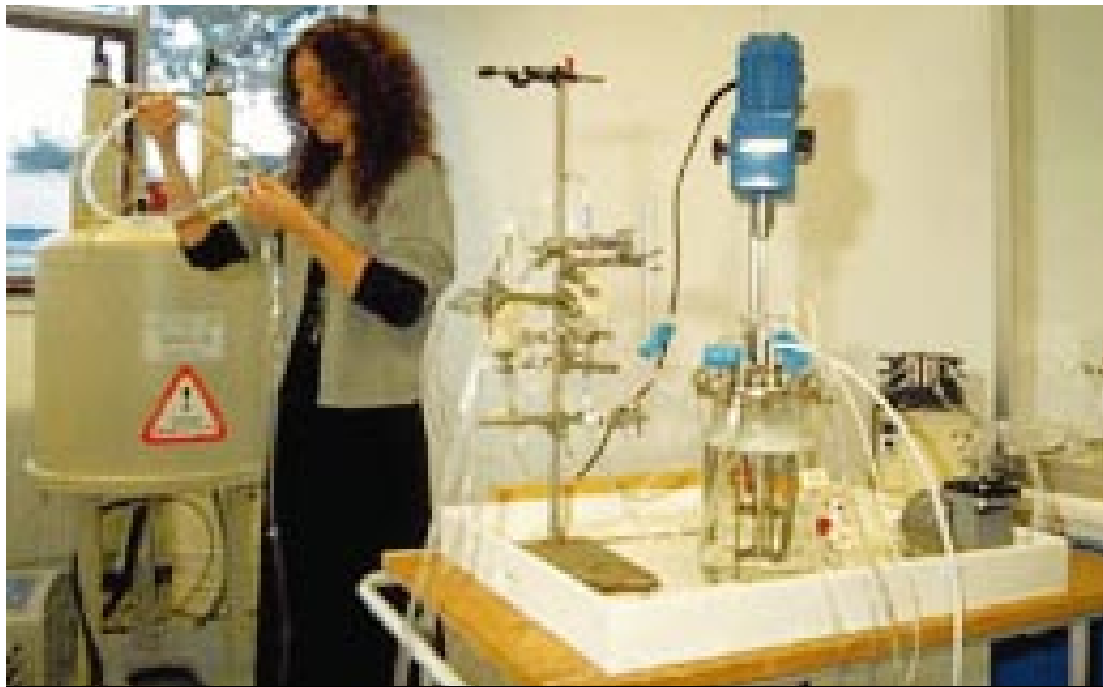
Equipment for NMR spectroscopic studies of nitrogen fixation in living plant-microbe symbioses. The research is being undertaken by the Centre for Plant-Microbe Symbioses supported by the Danish National Research Foundation.
