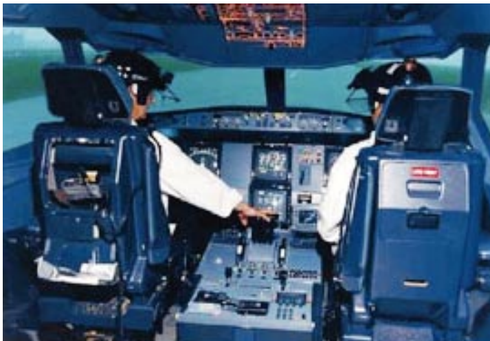
The Airbus 340 simulator at Aerospatiale, Toulouse, France. The pilots are wearing eye trackers during this experimental study of pilot behaviour during scenarios of abnormal take-offs. Risø was responsible for the experiment and subsequent analyses.
