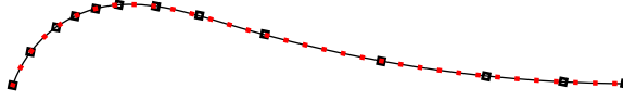
Figure 4.8.: Redistribution of the immersed boundary marker points □ redistributed point, ■ original marker point
