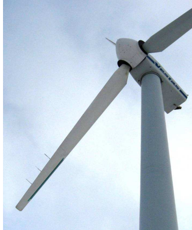
Figure 7.1.: ATEF turbine with active trailing edge flaps and Pitot tubes
