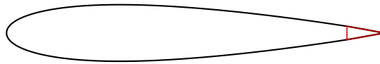
Figure 5.8.: Geometry of NACA0015 airfoil with a 10% flap represented as an immersed boundary (-)
