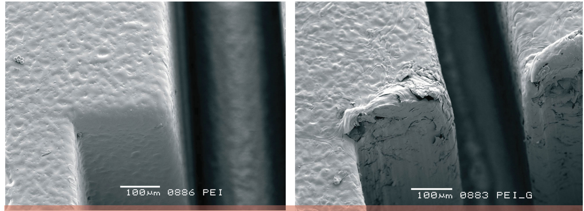
Figure 6: Effects of glass fibres on micro cracks of the injection moulded plastic parts (Part without glass fibre — left, part with glass fibre — right).
