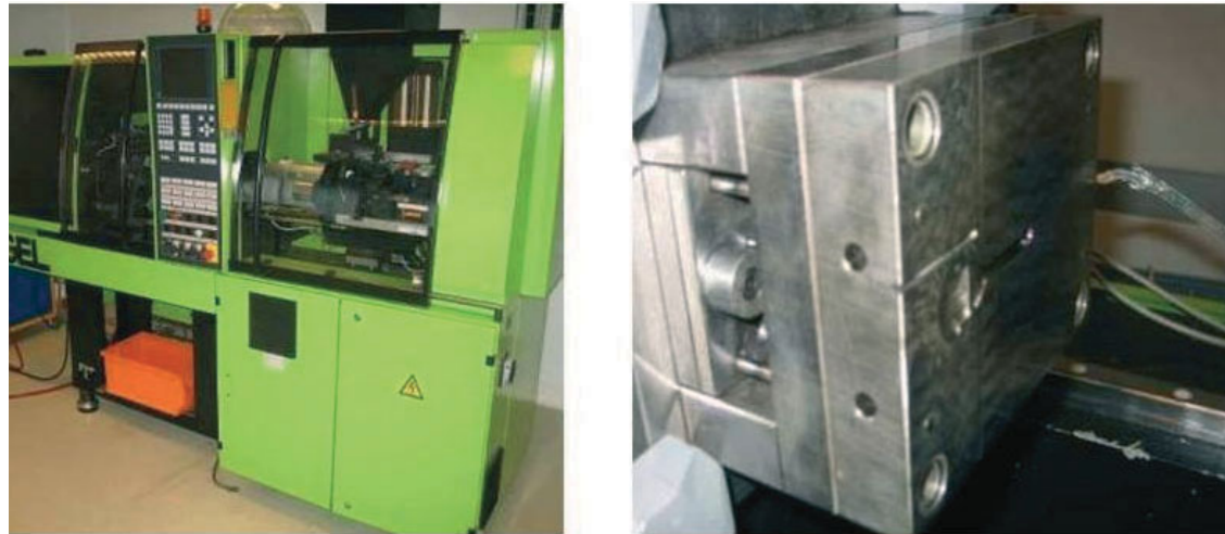
Figure 3: Injection moulding machine used for moulding of the plastic parts (left), and the moving side mould with cavity (right).
