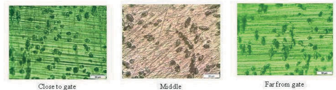
Figure 12: Cross section of glass fibre samples (Picture taken under the thin rib and at three different sections based on the distance from the gate location).
