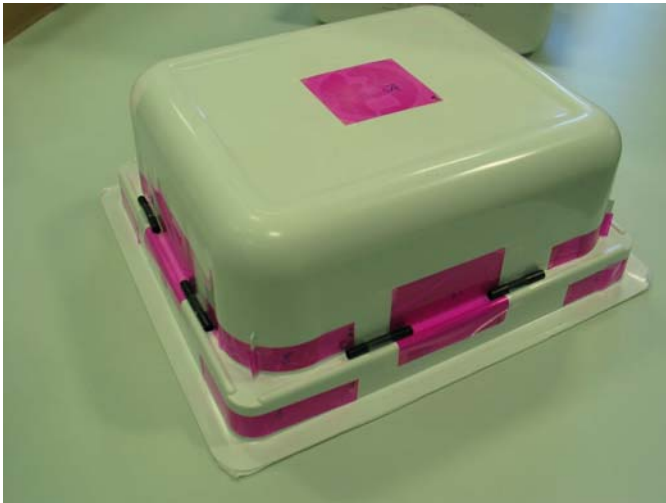
Figure 7. Complex product being dose mapped for sterilization at low-energy e-beam.
