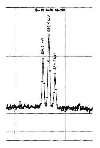
An obvious source of error would be a wrong value for our comparator standard. We store an aqueous solution with a concentration of 10 mg/ml of As, and its concentration was determined in 1966 not only by weighing the  $As_20_3$  to be dissolved, but also by subsequent chemical analysis. This analysis was now repeated, and a deviation of less than 2% from the original value was found.
