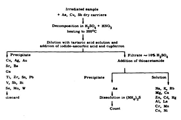
Our method is outlined on the first slide. After irradiation of the sample in the reactor, carriers are added, and the sample is decomposed in a  $H_2SO_4$ -HNO<sub>3</sub> mixture. We then perform scavenging, primarily to remove Cu and Sb, whereafter As is precipitated as sulphide. The precipitate is dissolved, and As-76 counted in a NaJ(T1)-detector. The chemical yield of the separation is finally determined by re-irradiation.
