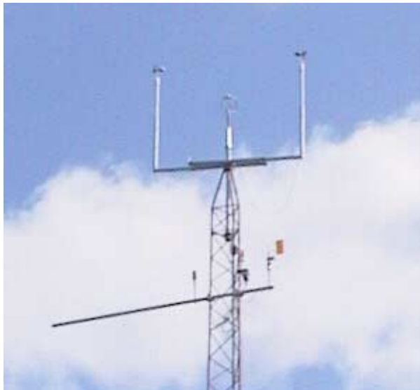
Figure 5-1 Anemometer comparison test setup with two RISØ P2546 cup anemometers separated 2m on a boom in the direction 15° to 195°, and with a sonic in the middle
