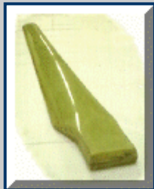
1.5 m long wind turbine blade produced in thermoplastic composites from the hybrid yarn.
