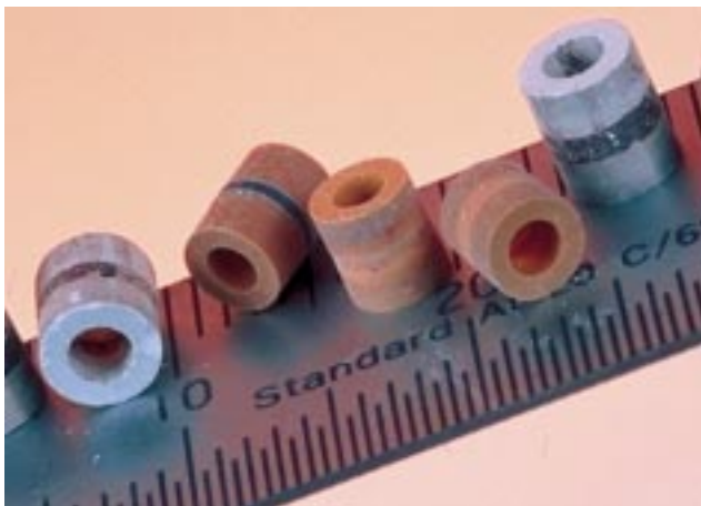
A cheap manufacturing method for electronic noise filters of functionally graded ceramics was developed in collaboration with AMP Danmark.
