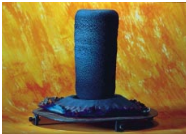
Top: The simulated build up of the material and the deposit temperature during spray forming of a rounded structure. Bottom: Spray deposited cylindrical structure (Diameter 8 cm, height 20 cm). The different shapes are obtained by variation of the spraying parameters.
