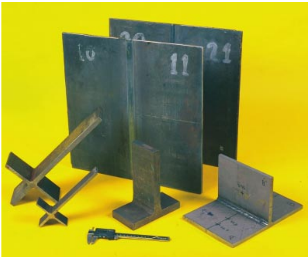
Residual stresses were measured by neutron diffraction in welded structures. The measured values agreed well with numerical predictions of welding induced residual stresses.
