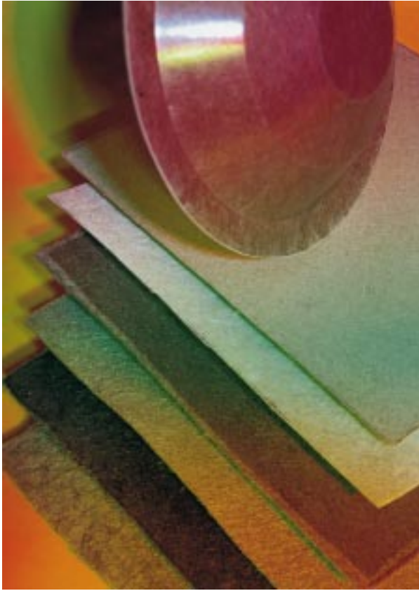
Three different types of semi raw materials based on natural fibres with the press consolidated laminate in between. Hemp is at the bottom, jute in the middle and wood fibres at the top. The hat shaped specimen at the very top is press consolidated from a jute fibre mat.
