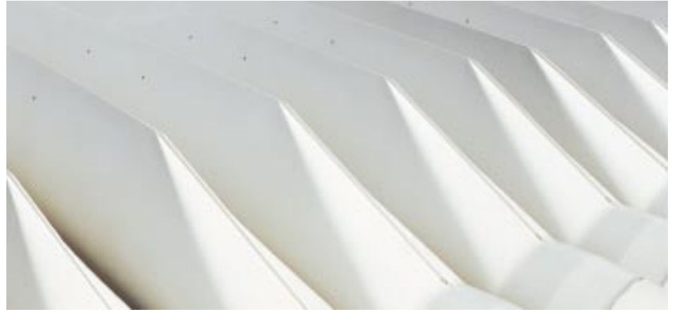
Wind turbine rotorblades produced by LM Glasfiber A/S. Stronger polymer matrix composites reinforced with carbon fibres are considered for large rotorblades.
