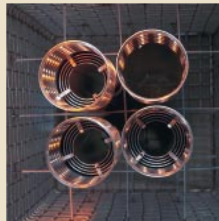
Four LEU elements. Each tube has a diameter of 10 cm and is 65 cm high.
