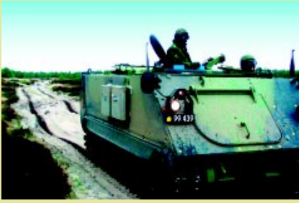
Two add-on armour panels are mounted on the side of an armoured personnel carrier (M-113) as part of a test run by the Danish Defence Research Establishment to investigate field conditioning of add-on armour. Similar panels are conditioned by the Department to compare the performance of field conditioned and laboratory conditioned armour.
