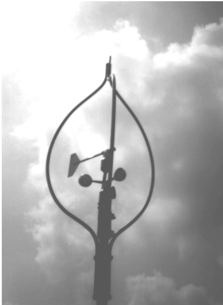
Fig. 2.4. Enercon nacelle anemometer with lightning protection
