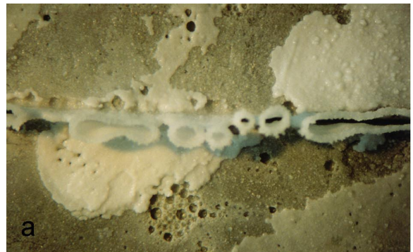
Fig. 3a Top of specimen 8-4 1 with calcite tubes formed from outflowing oversaturated solution.
