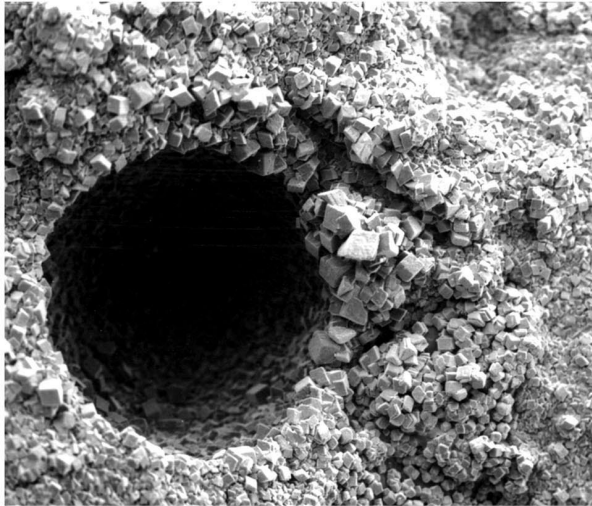
Fig. 4abc SEM (Scanning electron microscopy) of surface of calcite layers precipitated from synthetic \text{Ca}(\text{HCO}_3)_2 solution in cracks in cement mortar.
