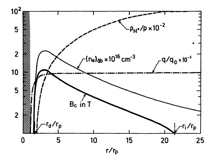
Fig. 4. Variation of the critical field,  $B_c$ , ablated electron density,  $(n_e)_{ab}$ , concentration ratio,  $\rho_H^+/\rho$ , and the energy flux ratio,  $q/q_o$  with the normalized expansion radius,  $r/r_p$ . Plasma state and pellet radius:  $T_e = 3.57$ keV,  $n_e = 3.38 \times 10^{13}$  cm<sup>-3</sup>,  $r_p = 1.31$  mm.
