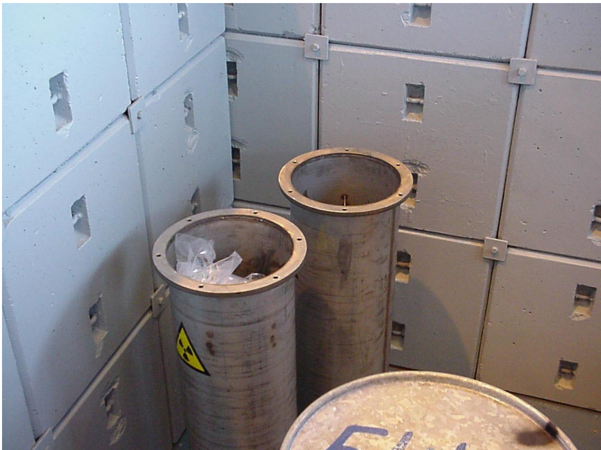
Figure A21. The two stainless steel containers for the beryllium reflector elements.
