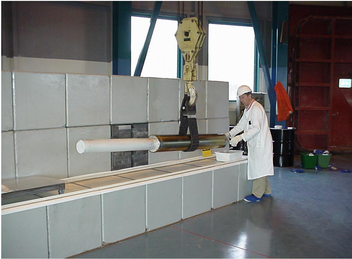
Figure A32. Measurement of the \gamma -dose rate along a beam plug.
