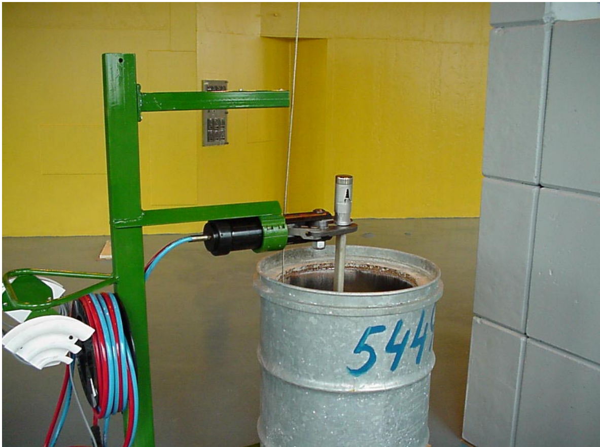
Figure A13. Cutting the armature and shock absorber off a shim-safety rod.
