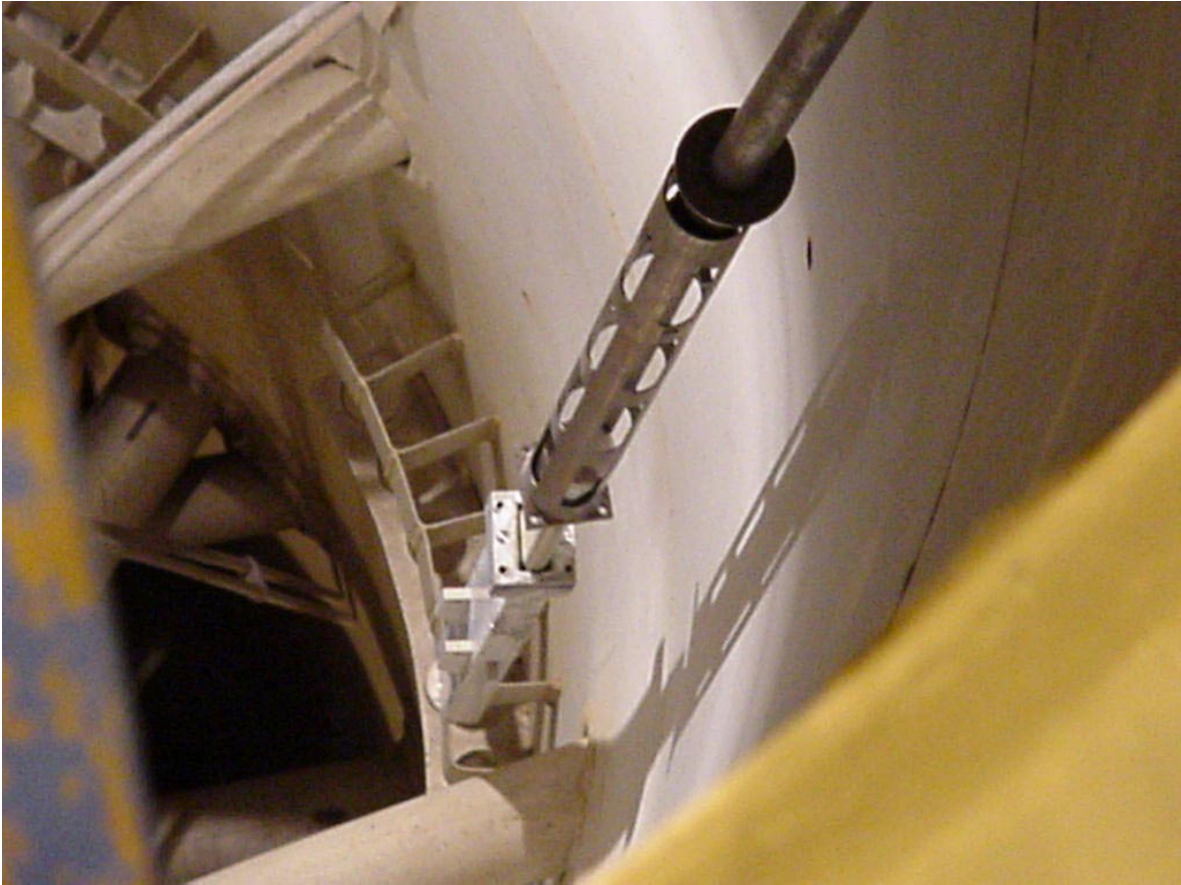
Figure A14. Calibration tool with stuck shim-safety rod and guide tube. Magnet rod on top.
