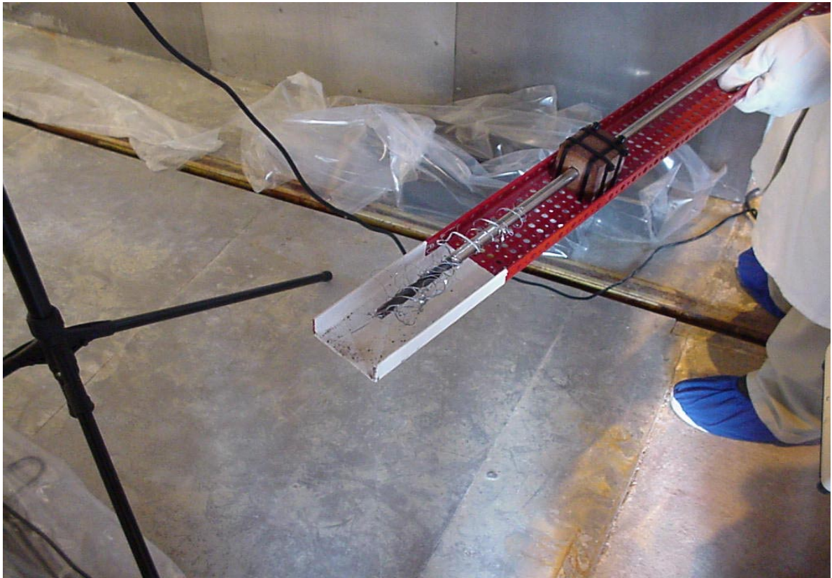
Figure A28. The drilling device for taking lead and aluminum samples at the wall at the inner end of the thermal column.
