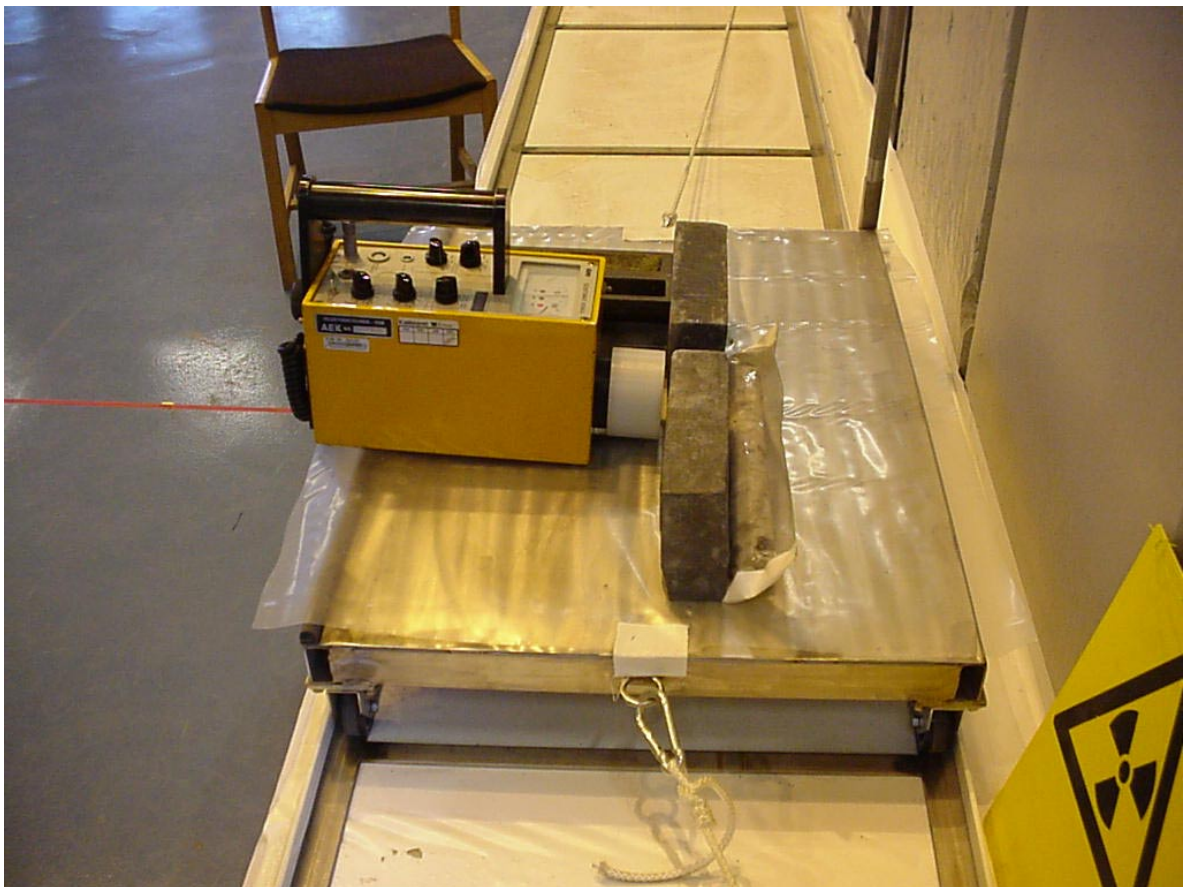
Figure A39. Measurement of the \gamma -dose rate along a borehole core.
