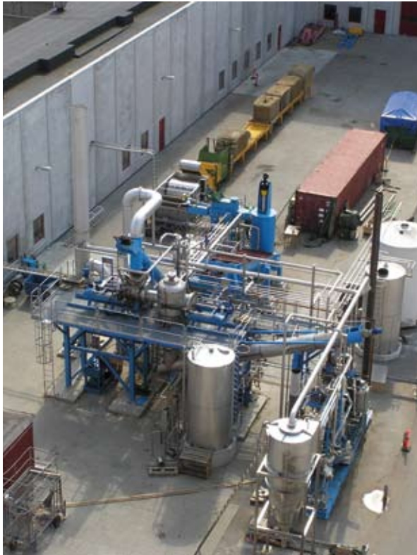
Figure 28. The Integrated Biomass Utilisation System (IBUS) for pre-treatment and processing of lignocellulosic materials can process 1 t straw/hour based on hydrothermal treatment. Photo: Elsam.
