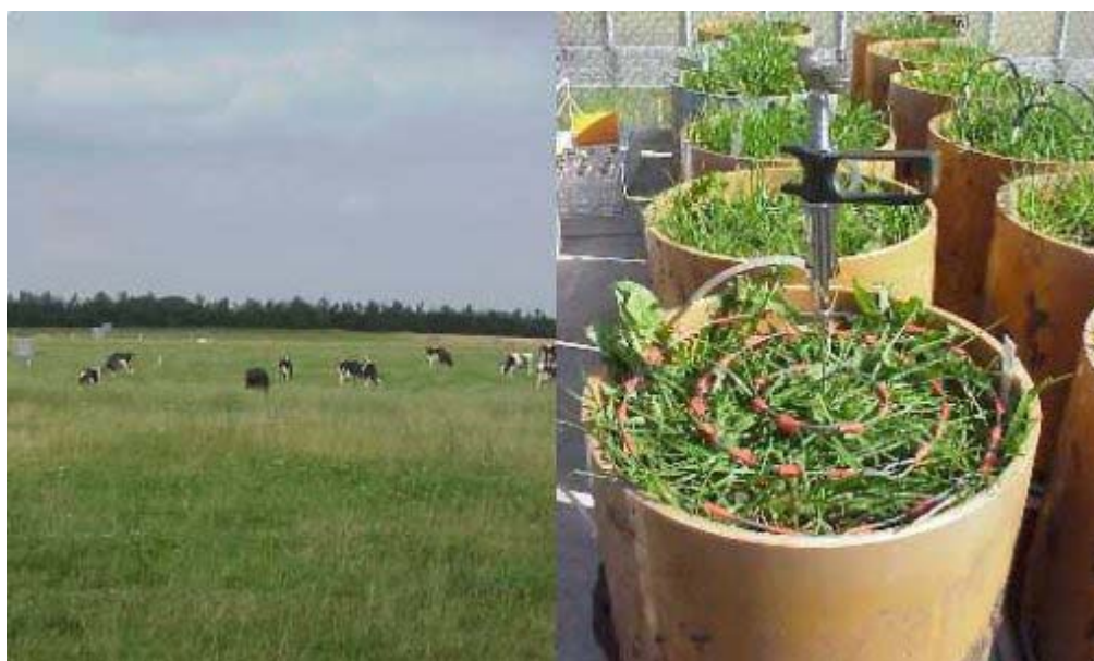
Fig. 3. Grass-clover monoliths incubated for ^{15}\text{N} -labelling and detection of \text{N}_2\text{O} emissions. The source of \text{N}_2\text{O} was investigated by cross- ^{15}\text{N} -labelling of the rhizosphere pools of \text{NH}_4^+ and \text{NO}_3^- combined with determinations of ^{15}\text{N} signatures of emitted \text{N}_2\text{O} (Fig. 3). The results show that \text{N}_2\text{O} is emitted simultaneously from both nitrification and denitrification independent of grass-clover pasture age (Fig. 4). The proportional contribution is seasonally dependent with nitrification being dominant in May and August and denitrification being dominant in June and October.
