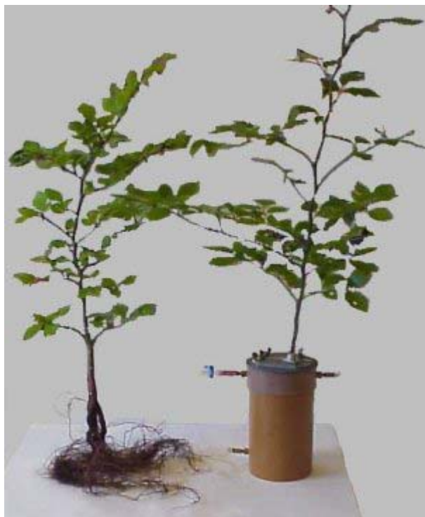
Fig. 2. Incubation of young beech plants for the determination of 13 C-signatures in CO 2 from root respiration.
