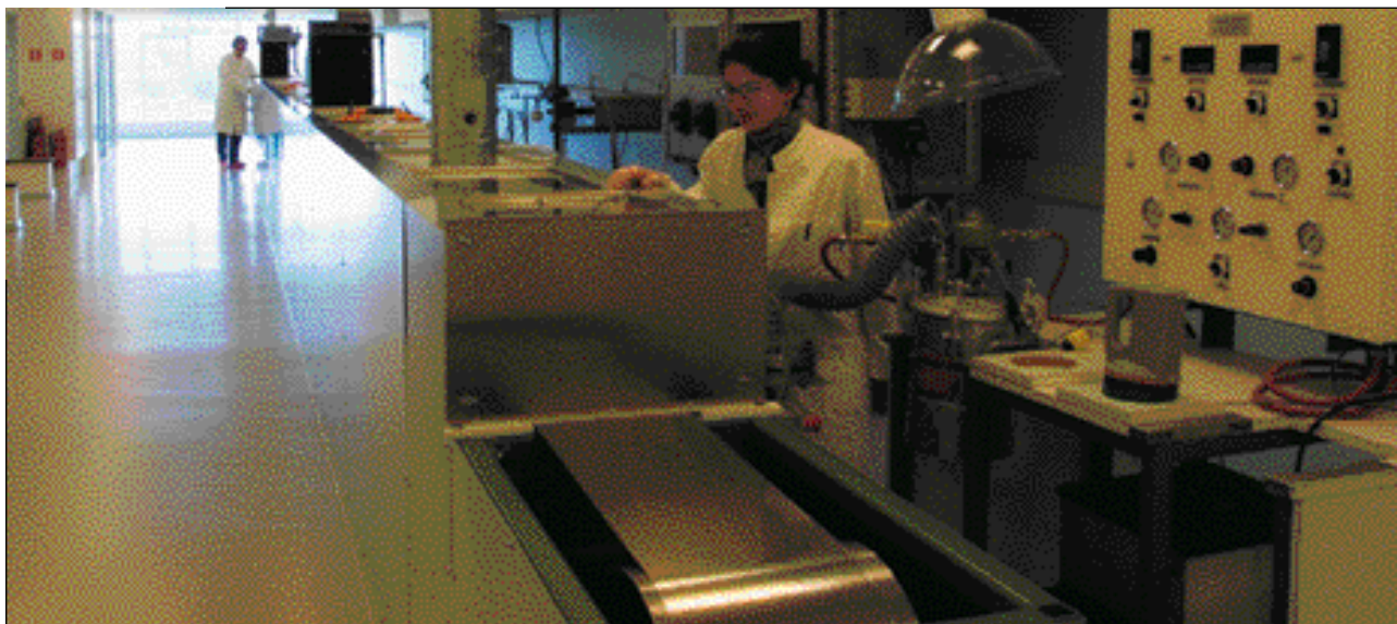
An experimental production plant for the manufacture of anode-supported cells has been established at Risø in collaboration with Haldor Topsøe A/S. The plant comprises a 20 meter long continuous tape-caster that is used for the production of anode supports.
