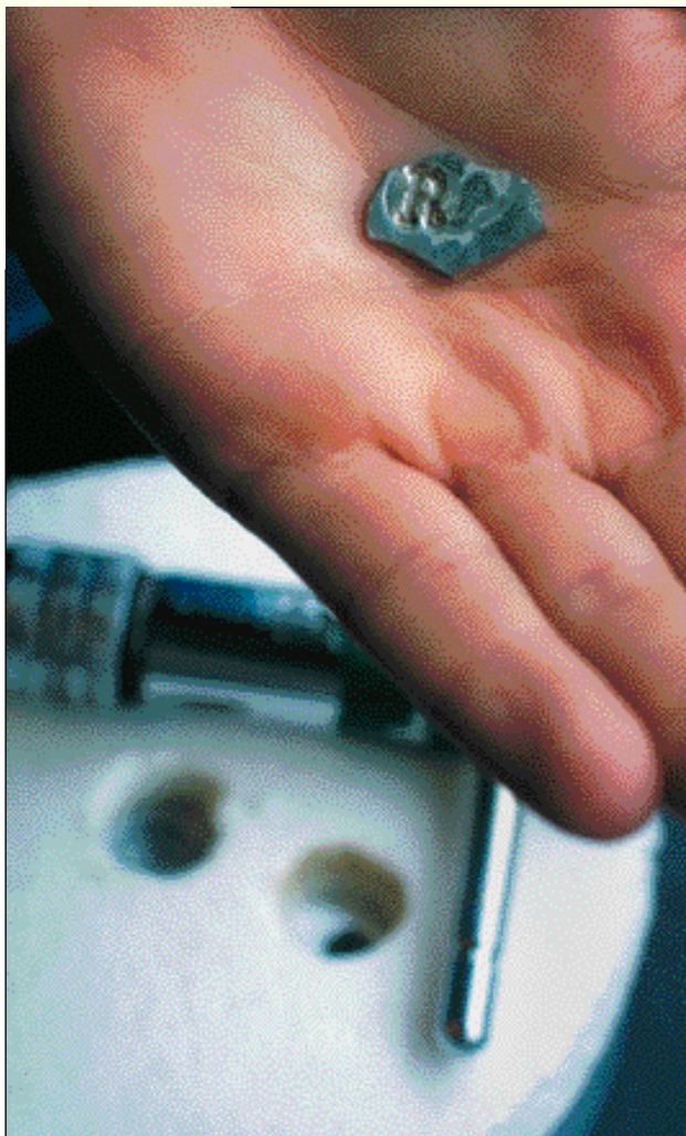
The subsequent impression is shown after cooling to room temperature. Only low forces are needed to shape the material and the amorphous properties are maintained.
