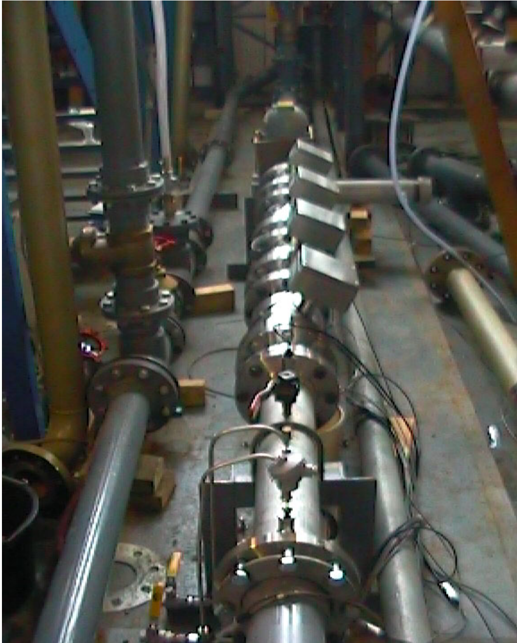
Figure 4.7: Picture of the horizontal test rig. The Gamma densitometer is on the far side.
