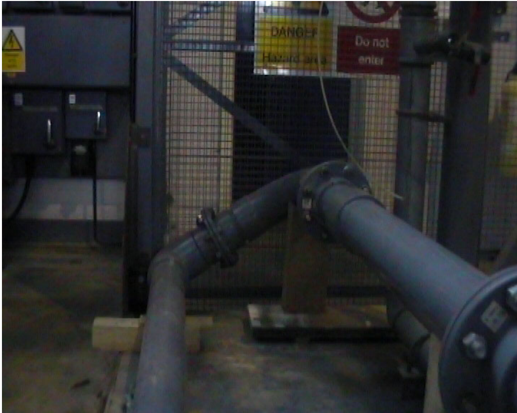
Figure 4.12: The small riser found at the inlet of the test section. This could be the cause for the small waves seen during stratified smooth flows.
