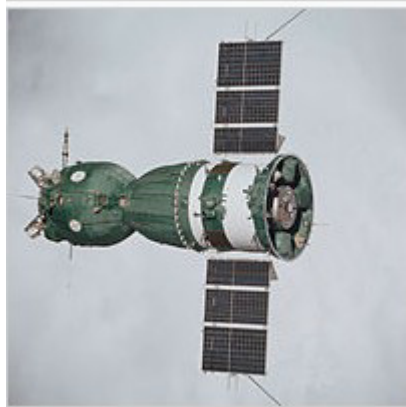
Figure 40. Soyuz 19 spacecraft for the Apollo Soyuz Test Project
