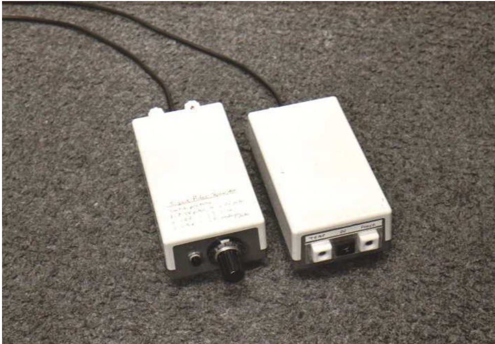
Plate 17. Load Cell Interface and Pulse coder (front views).
