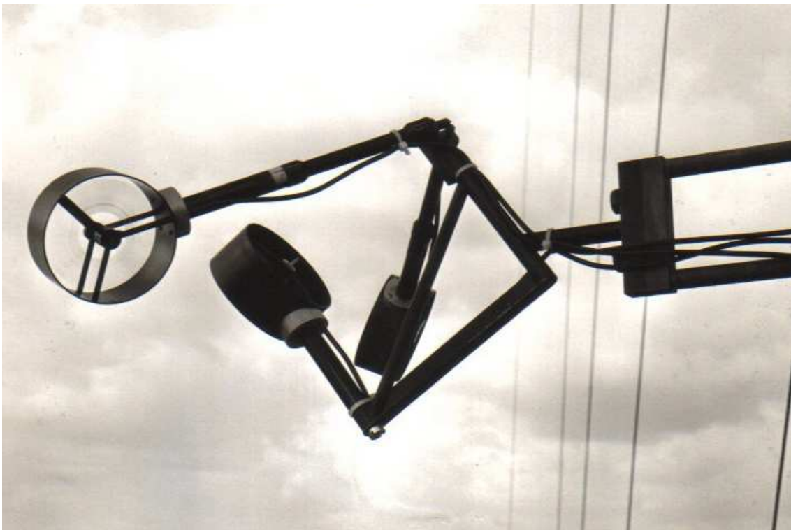
Plate 12. Non-orthogonal Digital Vane Anemometer triad.
