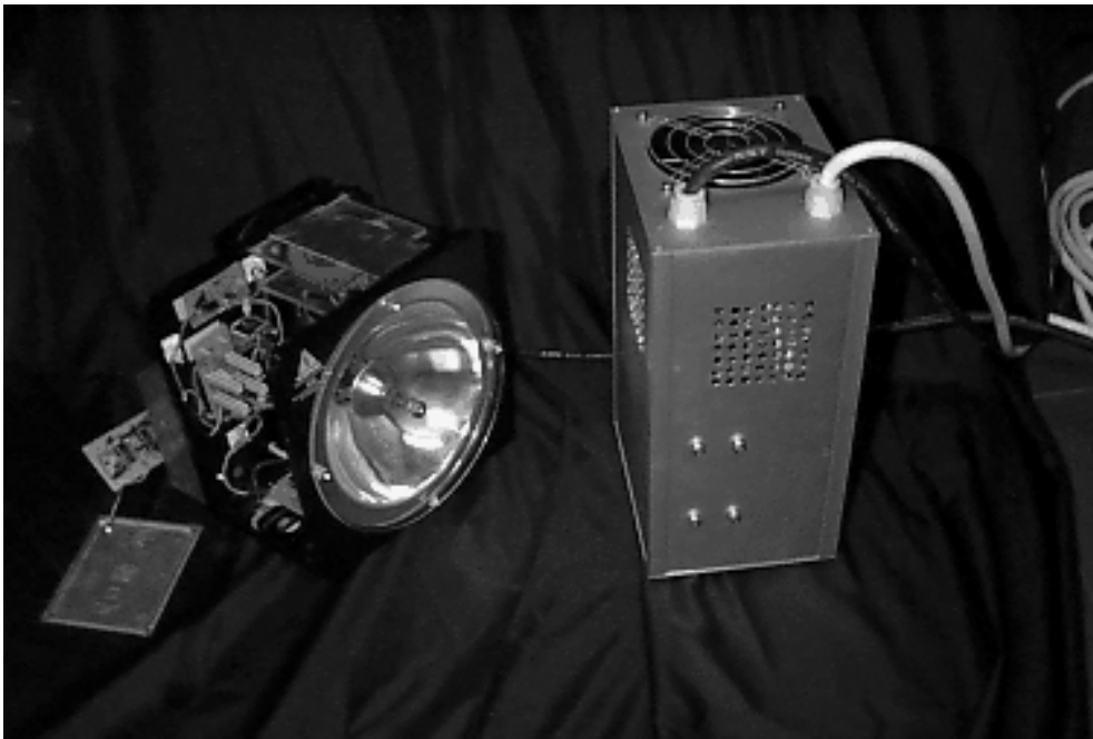
Figure 9. The rebuilt disco strobe together with its 500 V DC power supply.
