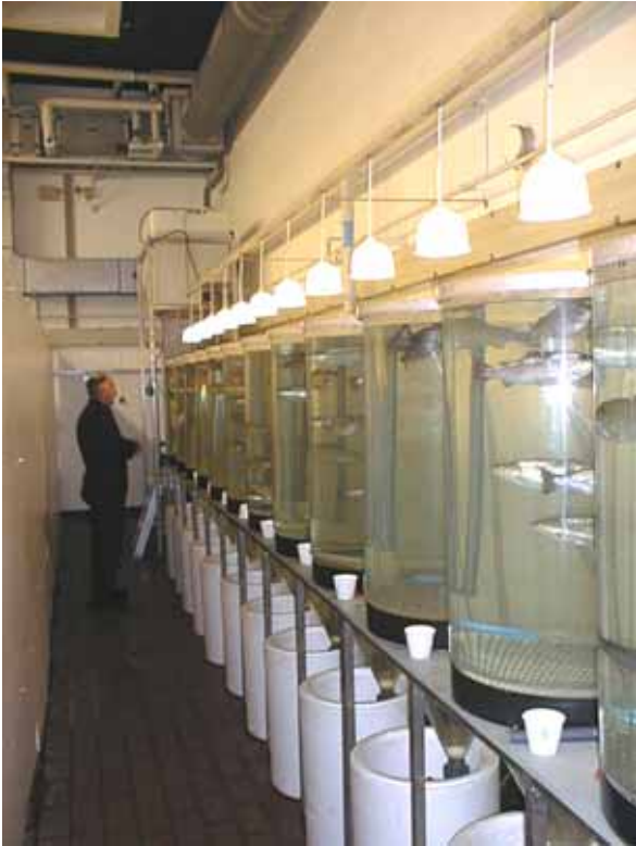
Figure 1. Experimental digestibility facility. 12 tanks for feeding and collection of faeces kept cool i.e. collectors submerged in ice-water, 0 °C in white polystyrene containers.
