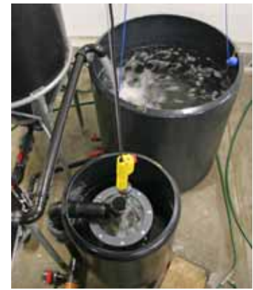
Fig. 2.4. Egg collector (bottom part of picture) and a reservoir (upper part of picture)
