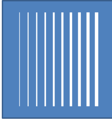
Figure 29. Schematic of the dose test pattern used, blue areas are exposed while white areas are not. The pattern contains 10 lines of ascending widths spaced 1 \mu\text{m} apart, with line widths ranging from 30 nm to 250 nm. The widely spaced single lines allow full AFM characterization, and the high area coverage requires very accurate proximity correction for the smallest lines to show up.
