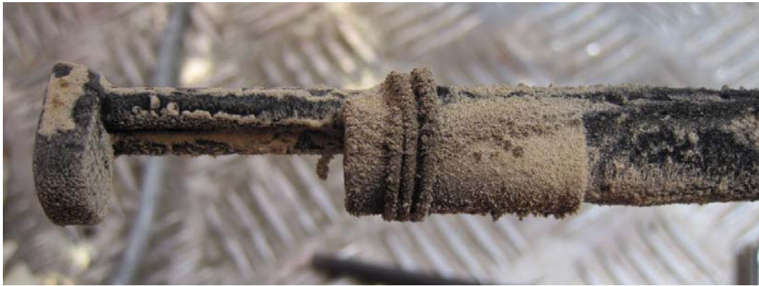
Figure 9 Deposits on FTIR-probe after measurements in the flame. The first layer on water-cooled stainless steel probe is soot (black areas). A simple wire supports the mounting of the ceramic tube on the probe. Optics is placed 20-30 mm inside the probe from the tip of the ceramic tube.
