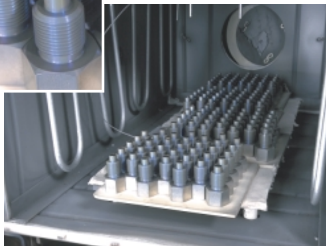
Furnace opened after brazing a charge of small nipples for Powder Technologies, Nordborg, Denmark. A silver alloy was used for brazing small ceramic ZrO 2 disks to (diameter ~ 5mm) the top of stainless steel nipples.
