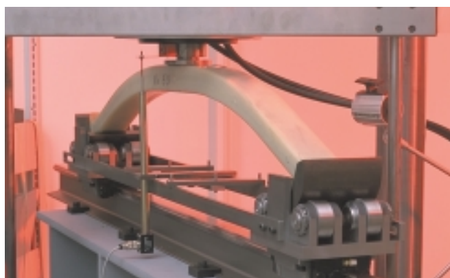
Testing of a 1.2 m long glass/polyester leaf spring for vehicle applications. The spring was manufactured by EM Fiberglas A/S.
