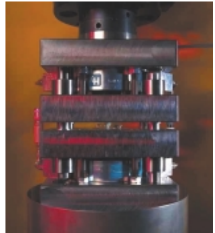
Test fixture (25 cm wide) for evaluating stiffness and compressive strength of thick laminates made by fibre reinforced plastics.
