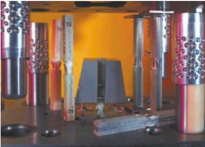
Test fixture (25 cm wide) for evaluating stiffness and compressive strength of thick laminates made by fibre reinforced plastics.
