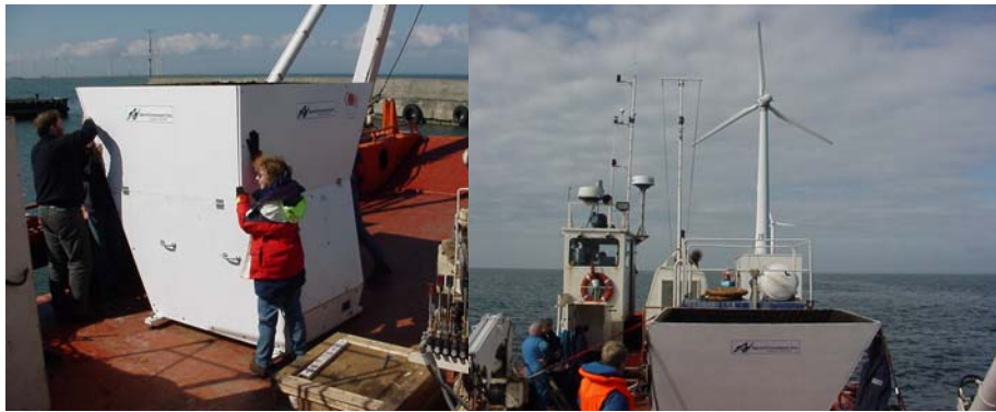
Figure 15. Setting up the sodar (left) and the sodar in position behind a wind turbine at Vindeby (right)
